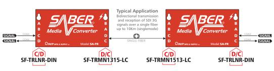
Kit consists of: SA-FR x2 SA-PS-NA x2 SF-TRLNR-DIN x2 SF-TRMN1315-LC x1 SF-TRMN1513-LC x1 D12PC-1-BLACK-BN x4 Optional Case: SK-A1400-BK
